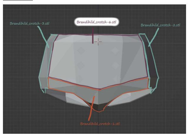
Glue or plastic weld the following parts together so they look like above. Please use flexible glue or plastic weld filler for this to ensure the seams do not break when flexing.
