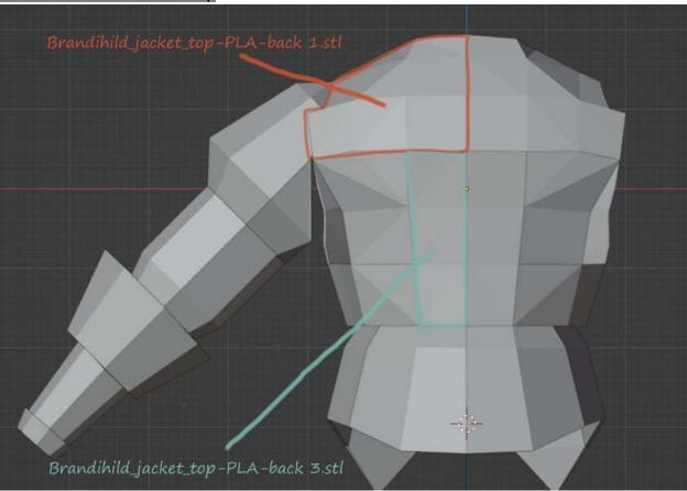
Glue or plastic weld the following parts together so they look like above. Using flexible filament to do a plastic weld here will increase comfort and durability.
