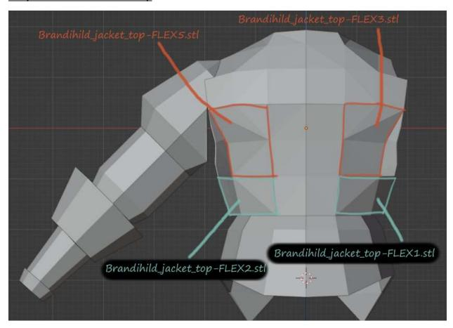
Glue or plastic weld the following parts together so they look like above. Please use flexible glue or plastic weld filler for this to ensure the seam does not break when flexing.
