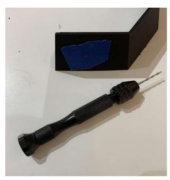
Before you drill the holes, put some masking tape over the spot you plan on drilling. That way you won't accidentally mar the paint surface while you work.
