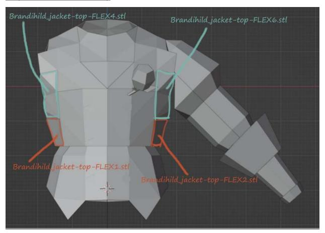
Glue or plastic weld the following parts together so they look like above. Please use flexible glue or plastic weld filler for this to ensure the seam does not break when flexing.
