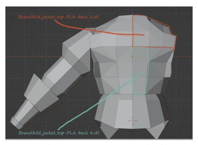
Glue or plastic weld the following parts together so they look like above. Using flexible filament to do a plastic weld here will increase comfort and durability.
