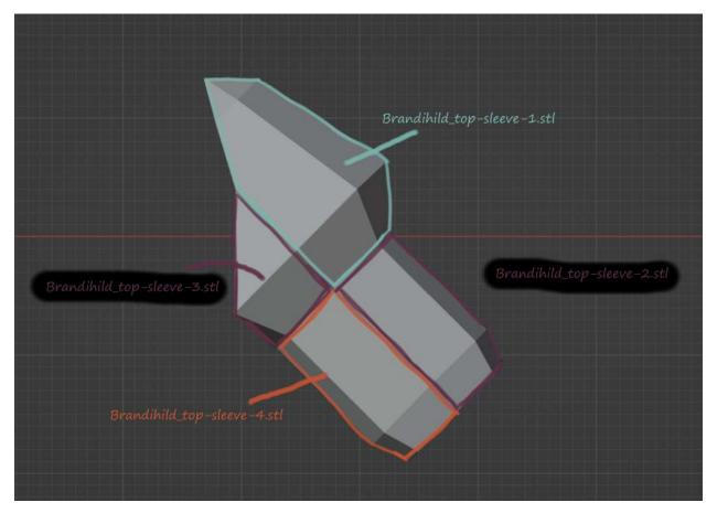
Glue or plastic weld the following parts together so they look like above. Please use flexible glue or plastic weld filler for this to ensure the seams do not break when flexing.
